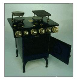
"The special feature of the Copeman oven is its automatic control. . . when the clock closes the switch, the current is applied just long enough to bring the food to a proper temperature . . . then the current automatically shuts off, but the dinner continues to cook without expense, the stored up heat in the oven and the heating element being sufficient for the purpose."
